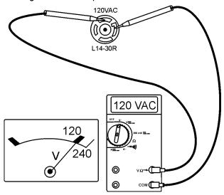
Figure 23. 120/240V Receptacle (120V)
